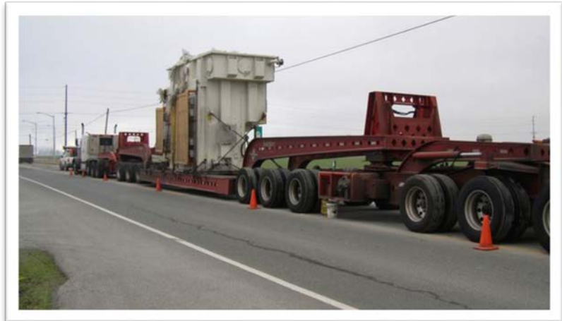
Example of a superload that would require bridge loading analysis.
